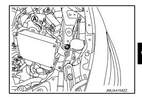
Remove washer tank inlet.
