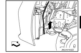
Remove washer tube from portion (A) of washer tank, and then pull out washer tube from clips (B).
