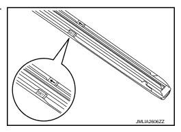
Pass through pawl of wiper blade in the groove of wiper refill.NOTE:
