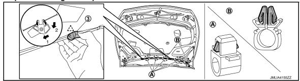
Pull out washer tube from fender gap, and then remove washer nozzle, washer tube as a set. CAUTION:
